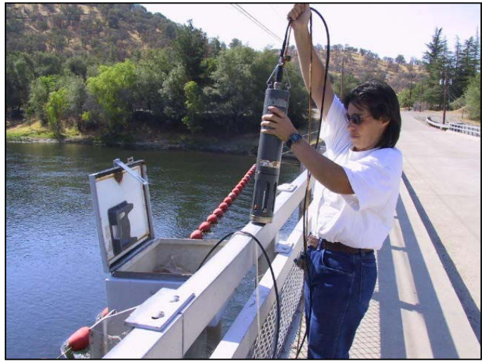
Figure 3-5. Dissolved oxygen monitoring station on the ACOE Bridge.
