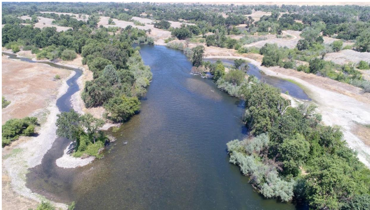
Figure 52. Examples of side channel (left of image) and floodplain (right of image) creation for juvenile salmon habitat on the Merced River, CA. The side channel has shallower depths and higher velocities compared the floodplain that has moderate depths and relatively low velocities.
