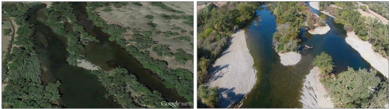
Figure 51. Example of riffle-pool creation on the Merced River, CA. The left image shows the pre-project channel, which consisted of mostly overly deep and coarse channels. The right image shows post project conditions after augmented gravels were placed to create several riffle-pool units with lateral bars and islands.
